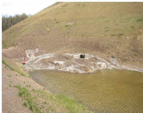
1. Efflorescent mineral bloom (white patches) at base of Siebert Waste rock site, adjacent to Siebert Pond, after prolonged dry spell.
