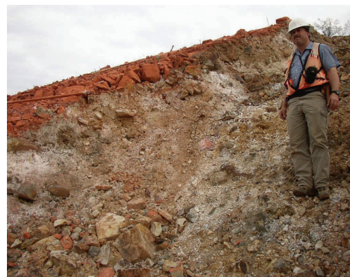
3. “Buttress fill” trench showing limited penetration of bauxsol (red) slurry over white efflorescent minerals (including green rust and gypsum) in layers of “baghouse lime”, and sulfate encrustations.
