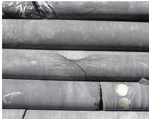
Appalachian Basin Black Shale Group core from the Marcellus Formation of central Pennsylvania. This core has been tectonically deformed as indicated by the vertical fibrous growth on pyrite nodules, tectonic cleavage wrapping around a concretion, and a calcite-filled fault zone
